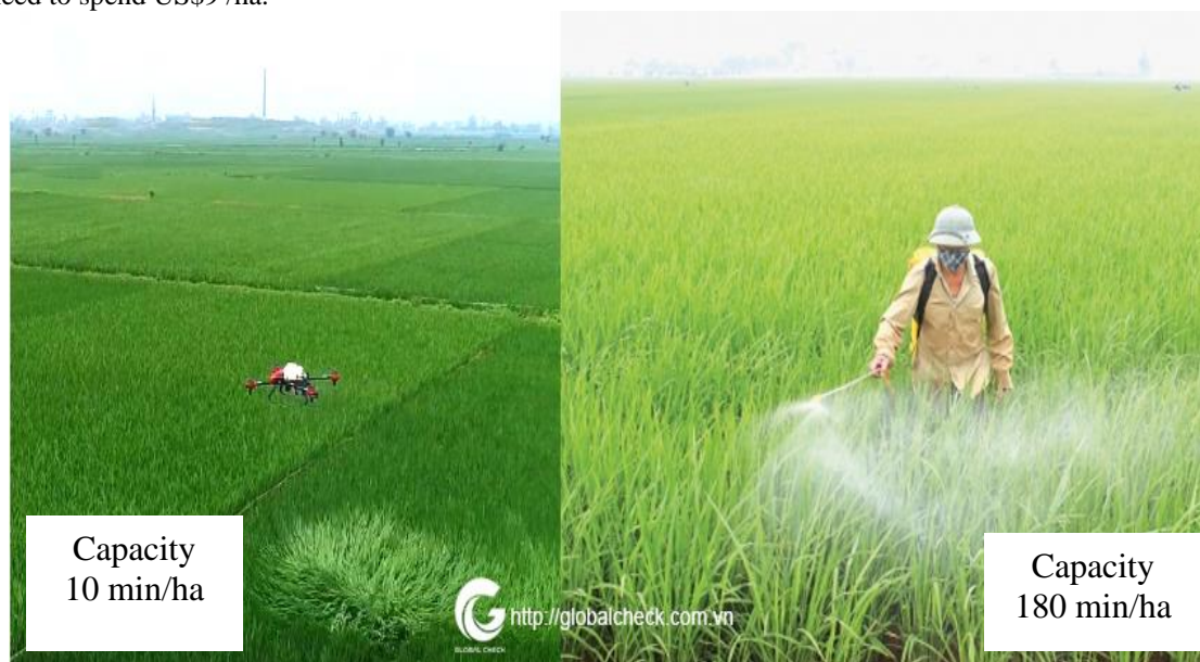
Figure 2. Drone technology to spray pesticides for rice paddy
