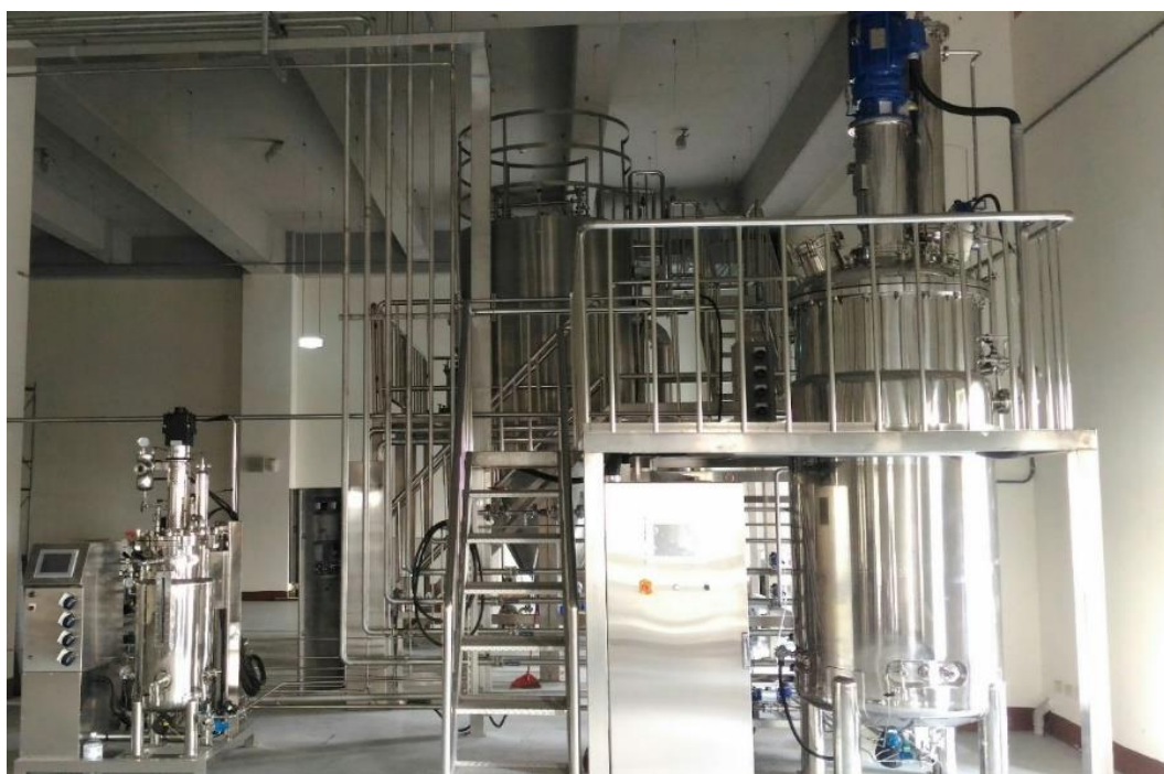
Figure 1. 100 L fermentation (left) and 1,500 L mass production fermentation tank (right).
