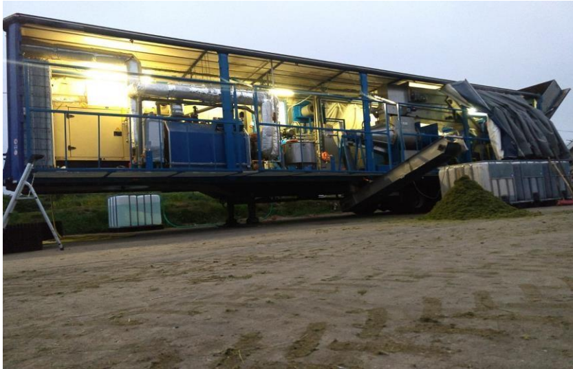
Figure 3. The 2 ton/hour Grassa mobile biorefinery
